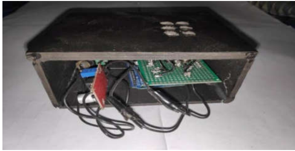
Fig. 5. Inner view of the braille display module
